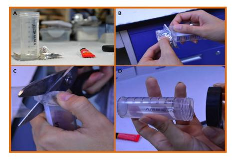
Figure 2. Finalizing the flyhandling and -collection chamber. (A) Once the glue is dried and the fine mesh firmly attached, (B) carefully remove the aluminum foil and (C) cut any excess mesh to conform the shape of the tube. (D) Here we used a custom-made plastic base on the tube, but you can use a small Petri dish bottom. Make sure the upper mesh is secure and that no holes are left where flies could escape.
