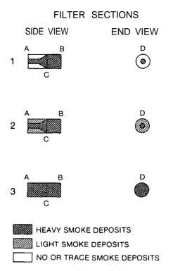
FIGURE 1 - shows the progressive staining of the proximal end (A & D) of the filter downstream from the perforation line (C) as the number of holes blocked increases from one in filter 1, to a partial block in filter 2, and a complete block in filter 3. B is the distal end of the filter. Kozlouski et al. 1980a. © 1982, American Public Health Association. Reprinted by permission.
