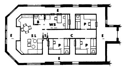
FIGURE 6. Diagrammatic representation of the overall floor plan of the laboratory and its arrangements within the external building shell.
